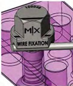
**WIRE FIXATION BOLTS** are made from stainless steel. A tight tolerance shoulder is designed to distribute the bending load of the bolt when being tensioned. The bolt offers a serrated 2.0mm wire v-slot to keep the wire from loosening. The top of the bolt is marked with a black line across the top indicating the location of the wire slot. The bolt has a 10mm hex head allowing more wrench placement for counter-torque.
